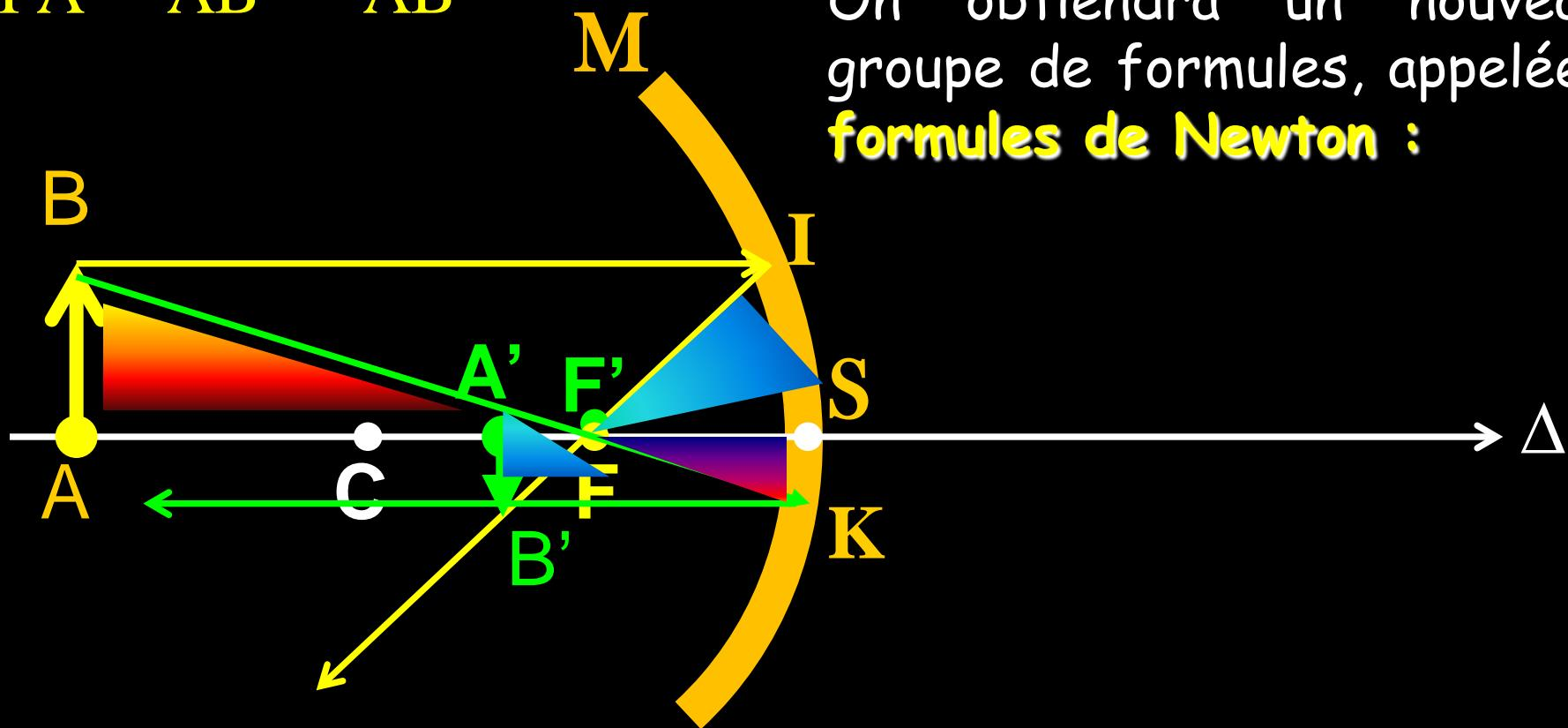
$$\frac{\overline{FS}}{\overline{FA}} = \frac{\overline{F'A'}}{\overline{F'S}} \Leftrightarrow \frac{\overline{FA} \cdot \overline{F'A'}}{\overline{FS} \cdot \overline{F'S}} = \frac{\overline{FS}}{\overline{FA}}^2$$
