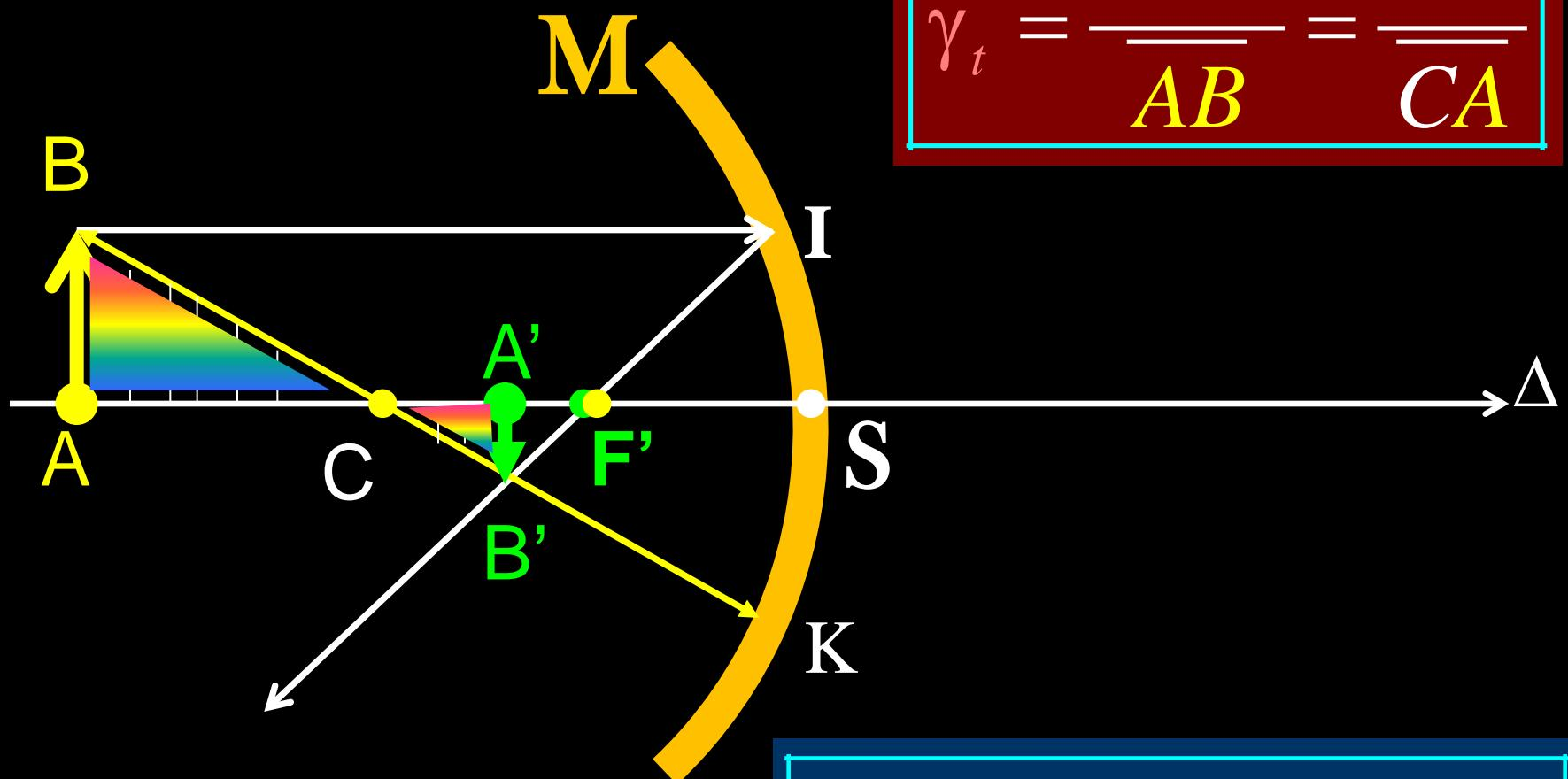
$$\gamma_t = \frac{\overline{A'B'}}{\overline{AB}} = \frac{\overline{CA'}}{\overline{CA}}$$
